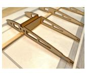
Locate one R2 from BP5. Glue it in place as shown, making sure the tabs from both SW2s are fully inserted. Also make sure that R2 is perfectly aligned at 90° to the building surface.
