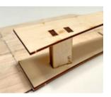
**Step 68 - Fuselage - FS5** Locate two FS5s from BP3. These are glued together, stacked on top of each other, then glued in place as shown here, just forward of F2A/B.
