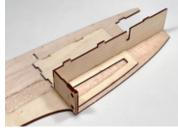
making sure you know how all the tabs/slots fit together. This is where the extra long tabs on the lite-ply parts will aid in getting the proper alignment to the sheeting.
