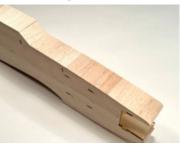
grain is cross-ways. Mark, cut and glue a portion of the sheeting in position. Repeating this technique, work your way forward to the nose.
