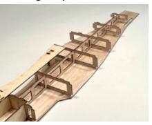
When you're satisfied on how this goes together, remove the spine, apply glue to the outer edges of F4 and F5, as well as the portion of F9 that runs from F5 to F3. Glue this in position making sure it's firmly inserted in all the above-mentioned places.
