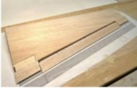
**Step 34 - Wing - R1** Now it's time to cut a square hole out of the root rib (R1). This will be between the precut slots for the sheer webs and between the upper and lower spars, as shown here.
