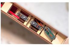
wings to get the servos, extensions, and pushrods in place. Shown in the following photos are an examples of the radio gear's installation in one of the Fifty-One prototypes. Take a bit of time to plan things out
