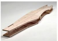
satisfied with the fit, remove the sheeting and apply glue to the outer edges of the formers and plywood structure.
