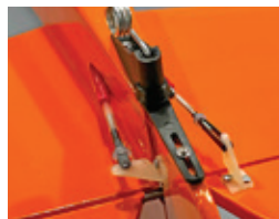
Typical aileron pushrod install on the left.
