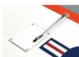
Typical aileron pushrod install on the left.
