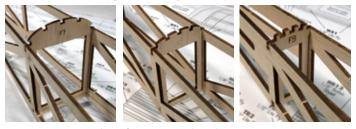
Locate F7, F8 and F9 from BP1. Glue these in position one at a time, working towards the rear. Make sure to evenly squeeze the fuselage sides together. This will keep the fuselage straight and true.
