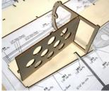
Step 46 - Fuselage Assembly (TR2 installation)
