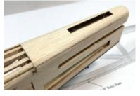
extends into the wing saddle. Also take the time to round off F10 so it matches the slope and curvature of the stringers.
