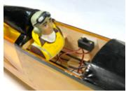
one of Horizon's 1/7th scale pre-painted pilots. Using a bit of the leftover wood, you can easily make a shelf where you can mount the pilot. Make sure his head is at the right height to rest level with
