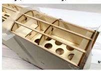
leftover  $1/8" \times 1/8"$  balsa strips to span between F3 and F2 while resting on the fuselage sides. Position H1 up against the back of F2, resting on both of the 1/8" square strips. Now position H3 against the front of F3, again, resting on the 1/8" strips. When satisfied that everything is properly positioned and lined up, glue these pieces together.
