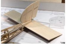
time to make sure these glue joints are sufficient, but don't use too much glue as it will make the Sky Ranger unnecessarily tail-heavy.
