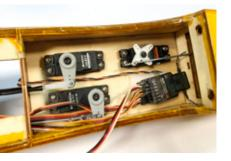
Make sure that when installing the control horns, they are placed in-line with the pushrods, and that the line of holes where the clevises attach are positioned over the hinge line.
