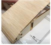
hinge allowing you to put a small amount of adhesive in the joint. When the adhesive is applied, place the sheeting back down on the waxed paper, so that it's flat (as shown in the photo). When cured, you'll now have a single, longer piece of sheeting.
