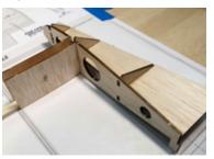
rest flush on the building surface - just as shown in the photo. This will insure a proper 90° angle for R5. Also make sure that the bottom edges of both WB2s are properly glued to the bottom spar.
