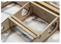
the slots. They should *not* be flush with the outer rib surface. Also cut a length of leftover cap-strip to span the R4 ribs. It will fit in the notch just behind the rear hatch mount. Glue in place.
