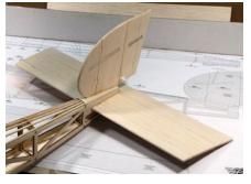
time to make sure these glue joints are sufficient, but don't use too much glue as it will make the Sky Ranger unnecessarily tail-heavy.
