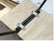
Place the two of the included nylon landing gear straps in position, then mark and drill 1/16" holes where the straps
