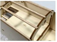
Using the leftover  $1/8" \times 1/8"$  balsa from the previous step, measure, cut and glue the front stringers that run between F4 and F3.
