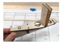
butted up against R5 and at a 90° angle. Now place a few drops of thin CA in the joint. It will cure in just a matter of seconds, holding it in place. Do the same for the other WB2.
