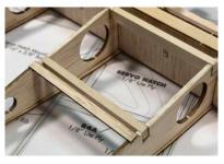
the slots. They should *not* be flush with the outer rib surface. Also cut a length of leftover cap-strip to span the R4 ribs. It will fit in the notch just behind the rear hatch mount. Glue in place.
