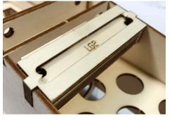
installed in the fuselage one at a time and laminate together to form a sturdy block for the landing gear wire.
