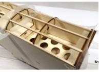
leftover  $1/8" \times 1/8"$  balsa strips to span between F3 and F2 while resting on the fuselage sides. Position H1 up against the back of F2, resting on both of the 1/8" square strips. Now position H3 against the front of F3, again, resting on the 1/8" strips. When satisfied that everything is properly positioned and lined up, glue these pieces together.
