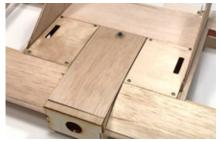
When in place, use a 1/16" bit to drill through the 4 pre-cut mounting holes in each hatch, into the 1/4" basswood underneath. Later on, you can use the supplied  $2-56 \times 3/4''$  self tapping screws to hold these in position.
