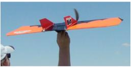
to what's shown here - by the skid, throttle up, then throw the Bat forward and just slightly nose-up. **And I do mean slightly - not 45°**.
