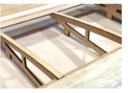
centered on the rib and run from the rear of the leading edge sheeting to the front of the trailing edge sheeting.
