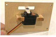
1/4" wider than the servos you are using. Glue two pieces together to form 4 mounting rails. Lightly sand the ends of the rails to true them up.
