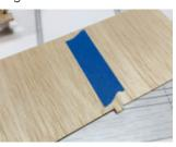
hinge allowing you to put a small amount of adhesive in the joint. When the adhesive is applied, place the sheeting back down on the waxed paper, so that it's flat (as shown in the photo). When cured, you'll now have a single, longer piece of sheeting. You'll need to join a few pieces together to make it long enough to
