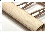
the wood to expand the fibers. Now hold it to curvature needed, then use a hair dryer or covering heat-gun to help "set" the balsa's bend as it dries. Once dry, the you can glue it in position.
