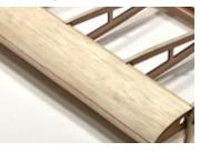
the wood to expand the fibers. Now hold it to curvature needed, then use a hair dryer or covering heat-gun to help "set" the balsa's bend as it dries. Once dry, the you can glue it in position.
