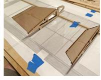
Apply a little glue inside the rib's pre-cut squares and just a touch on the bottom of the rear standoff.
