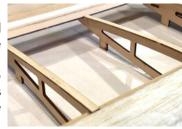
centered on the rib and run from the rear of the leading edge sheeting to the front of the trailing edge sheeting.
