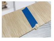
hinge allowing you to put a small amount of adhesive in the joint. When the adhesive is applied, place the sheeting back down on the waxed paper, so that it's flat (as shown in the photo). When cured, you'll now have a single, longer piece of sheeting.
