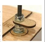
allow the bolt to turn in the hatch freely, and without a lot a slop. Now thread on one of the 4-40 lock nuts all the way to jam against the 4-40 nut previously installed.
