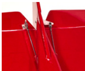
Typical elevator and rudder pushrod setups.
