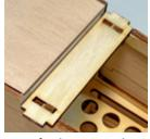
When you've done that, you can then test fit the H2 and H3 assemblies in their proper spot and make sure they fit somewhat snugly. Lightly sand as necessary to get a proper fit. BUT STEP AWAY FROM THE GLUE BOTTLE. DON'T PUT ANY GLUE ON THESE, or it's gonna be trouble.
