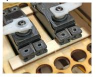
Then this assembly can be glued to the top of TR2, with the tabs fitting inside TR2's circles (again, only fitting properly in one way). Before gluing this in place, we chose to install the ESC on TR2 first, then installing the TR4 tray.
