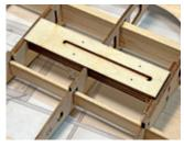
slot will align with the hole in LG2, only if correctly positioned. When you know how it correctly aligns, apply glue to the back side of LG1, then glue it in position, making sure to keep excess glue out of LG1's slot.
