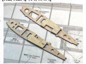
(towards the wing root). When glued in place, R2A and R4A need to be perfectly aligned with top and bottom edges of their respective ribs. Also the rear edge should be just on the edges of R2A and R4A should be aligned with the rear spar cutouts in each rib.
