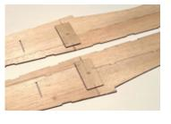
they will only align properly one way (FS5 port, FS6 starboard). When satisfied on how they align, glue them in place to the fuselage sides.
