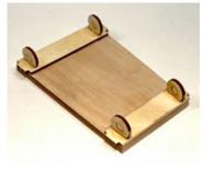
When satisfied with the fit of H1, put a few drops of glue on the top surfaces of H2 and H3 (which should have been sitting in the fuselage this whole time). Then press H1 down onto these pieces,
