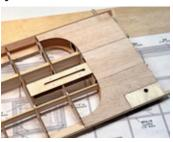
Also note that CS6 has a pre-cut hole in it. This is where the wing bolt will go through to attach the wing later on. This hole should be positioned so it's closer to the root rib (R1). When this assembly is completed, glue it in place using the same techniques as applying the top sheeting.
