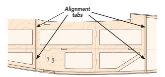
Step 52 - Fuselage Assembly (port & starboard sheeting)
