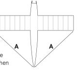
When the wing is aligned, use a pencil to transfer the wing's bolt holes through to WH1/WH2 already installed in the fuselage.
