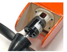
mount also has down-thrust built into it. By using a couple washers between the mount and the firewall on the bottom two mounting screws, you can take out some of this thrust.
