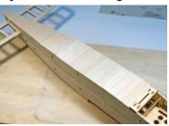
cut and glue the first 4" section of sheeting in position. Using this same technique, work your way backward 4" at a time, until you reach the rear of the fuselage. Be careful not to waste as little of the sheeting as possible.
