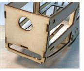
sanding is needed to bevel the sides of F2 to obtain a secure fit. F2 needs to be flush against the front of TR1, and the tabs from both fuselage sides need to be inserted into the pre-cut slots in F2. When satisfied on how these pieces go together, it's time glue things in place and we recommend using epoxy for this step for it's extra strength and working time.
