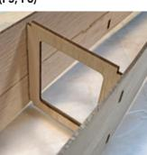
making sure that the rear fuselage sides remain aligned. Refer to the top view on the fuselage plans to see how the rear of the fuselage should be curved - symmetrically straight and true - not bowed to the left or right (banana shaped).
