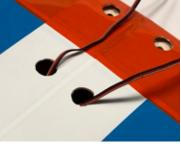
Cut into LP4 are SM3's (elevator, rudder and throttle, servo mounts).
