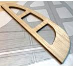
Step 37 - Vertical Fin (V1, V2) Glue the V1 and V2 assemblies together as shown here to form the completed vertical fin.
