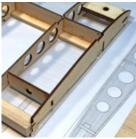
It's crucial that this part be glued in correctly and that it is glued with no warps or twists.
