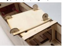
the top - test both ways for the best fit. When properly seated, it will fit in the area between H4 you just installed and F2. You may have to do a little sanding to get a good fit.
