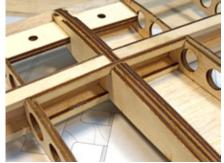
When properly aligned, there will be a slight bend at the center of the wing (dihedral).
