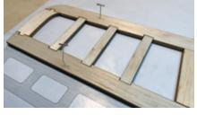
These are now glued in place as shown, making sure they are firmly seated in the pre-cut notches in S1 and S3.
