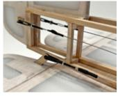
We used some of the leftover 3/16" sq. basswood to form the servo mounting beams inside the fuselage.
