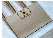
Step 43 - Wing Assembly (CF3) Locate CS3 from BP11. This is glued over the front part of the center section.
