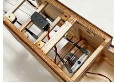
These photos shown examples of servo installation in one of the Minuette prototypes. As you can see, we've used Dubro's 2-56 pullpull setup for the elevator and rudder and it works very well. You can use other systems, but a pullpull system will look best as it's more "period correct".
