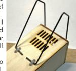
Using an 1/8" drill, clear out the two small pre-cut holes in the firewall. Then push the port and starboard struts completely into these holes.
