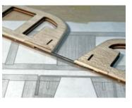
use a 5/64" drill to carefully open up the groove and remove any glue that may have seeped in. DO NOT CUT THROUGH THE OUTER SHEETING.
