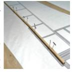
fuselage. Slightly bevel the pieces where they meet at this "break" for a good fit.
