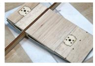
carefully work your way down to a proper fit by using a sanding block. Remember you can always take wood off, but it's a lot harder to put back on!
