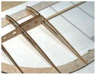
pieces fit, glue them in place, making sure they're aligned and all tabs are properly seated. The bottom edges of the SW4s should be glued to the sides of the lower spar and the rib should be flat against the plans.
