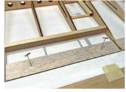
side of the R6 ribs. Pin this in position.
