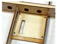
place on the plans, between the ribs and up against the lower spar. Now SW3 will be installed to form the 4th side of the aileron box. It should be snug up against both ribs, and loosely against SH1. I say loosely because you'll want to leave a touch of room to account for the thickness of covering to be applied later.
