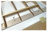
ribs already in place on the main wing (extending the look). Don't worry about the other two marked on the plans just yet.
