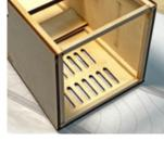
Make sure the fuselage sides are parallel in when doing this.
