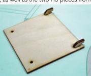
Carefully sand this to match, test fitting along the way. When satisfied with the fit, place the hatch over a small piece of wax paper, making sure that is upside down. Glue one H3 in each of the two slots on the rear of the hatch, making sure that the H3 pieces point towards the rear of the hatch as shown.
