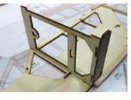
LG1 is slightly tapered, so when F3 and LG1 are glued in place, F3 will not be perfectly vertical. When satisfied with the location and fit of these pieces, glue into place on FRS.
