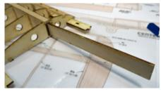
DH2's have a small circle engraved in them, and this circle should be positioned to the top and center of the wing.
