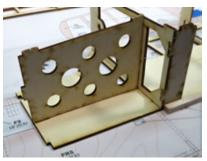
slots on FRS. TF must fit flush with the fuselage side, and former F3. When satisfied with the location and fit of TF, glue TF to FRS, but not to F3 at this time.
