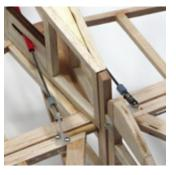
The flight pack battery is installed under the TF and the switch can be installed on the side of the fuselage where desired.
