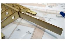
DH2's have a small circle engraved in them, and this circle should be positioned to the top and center of the wing.
