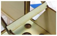
Once H5 is in place, H4 is glued to the back of H5, making for a stronger cross-brace.
