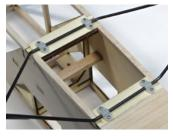
then mark and drill 1/16" holes where the straps should mount, then attach them using the supplied 2-56x3/4" self tapping screws.
