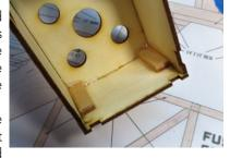
the fuse sides meet. The shorter pieces are used below F2. We recommend using epoxy to glue these pieces in.
