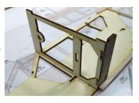
LG1 is slightly tapered, so when F3 and LG1 are glued in place, F3 will not be perfectly vertical. When satisfied with the location and fit of these pieces, glue into place on FRS.
