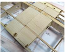
recessed slightly to allow this sheeting to fit flush with all the spars and trailing edge.
