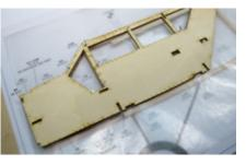
slightly longer than FRS around the firewall, to build in a bit of right thrust. Because of this, to properly line up FLS, use the window cutouts and the rear portion as reference.
