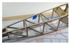
angles for a good fit. Pin these in position and glue into place.
