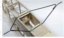
flux over the entire wire-wrap, then use a small torch (or a soldering iron) to securely older the wire wrap in position, securing the front and rear landing gear wires into a solid, one piece unit.
