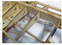
in step 30? Starting with the left wing panel, push the thread through this hole, then through the circular holes in R2, R3, and R4. The string will now extend from the servo bay, out through the bottom of the wing. Tape both ends of the string so they won't pull out. Do the same for the right panel.
