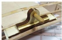
and WH4 from the LP4 sheet. Also, cut a 1-1/4" length from the included 1/4" dowel and round off one of the dowel's ends.
