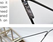
After cleaning, carefully and tightly wrap this joint with wire as shown here using. We used 26 gauge wire, but other thicknesses can be used. Starting on one side, lightly brush on a bit of
