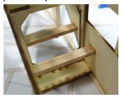
Step 77 - Fuselage Assembly (block sanding)
