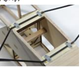
then mark and drill 1/16" holes where the straps should mount, then attach them using the supplied 2-56x3/4'' self tapping screws.
