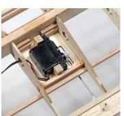
Now fit the servo hatches into position on the bottom of the wing. Using the pre-cut holes as a guide, drill four 1/16" mounting holes into the 3/16" x 3/8"basswood mounting strips installed earlier. Harden the wood with a bit of thin CA and you can use the attach the supplied 2-56 x 3/4" self tapping screws to secure them in place.
