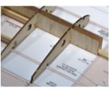
you will cut away the center of the R3 rib, leaving a box as shown in the photo. Then fit two of the WB3s in place. When satisfied with the fit and location, glue these pieces in place.
