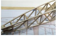
Step 74 - Fuselage Assembly (rear wing mounts - left)
