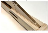
vertical fin. These strips should extend back to the cutout for the horizontal stab, as shown on the plans.
