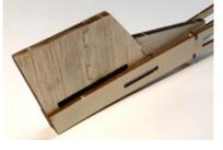
forward part of the fin will rest in the slot in the top of F6. When ready, remove the fin, apply glue, then put back in place, making sure that everything is held in place until the glue dries. It's best to do this on a flat surface to guarantee the fuselage isn't warped and the vertical fin is aligned absolutely vertical.
