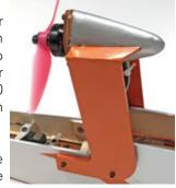
Shown here is an idea of how we mounted the motor in the prototype Wayfarer. The speed control was
