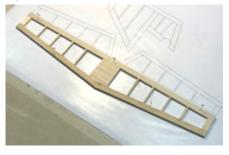
Once the glue has set, remove the finished stab from the plans and sand the leading edge to a round profile.
