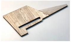
when satisfied, glue the pieces as shown to make the vertical fin. Sand the leading edge of VF1 and VF2 to a round profile.
