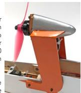
Shown here is an idea of how we mounted the motor in the prototype Wayfarer. The speed control was
