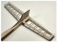
the fuselage. Adjust as necessary to make these measurements are the same. Also measure from each tip to the center of the fuselage's nose. These two measurements should also be equal. Once satisfied with the alignment, glue the stab to the fuselage.
