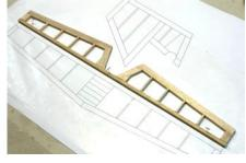
Carefully measure, cut and fit the pieces, gluing them in place as shown.
